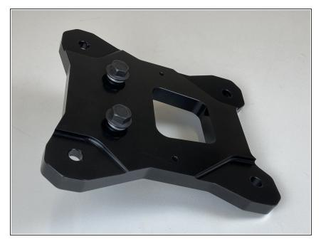
IMAGE 1 Assemble the new gusset plate by using the supplied bolts and lock washers along with an 18mm socket or wrench. Ensure lock washers are completely compressed.
