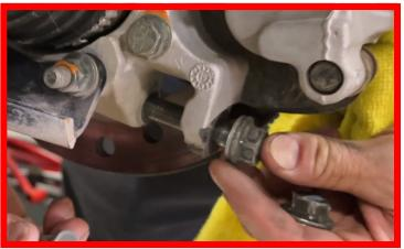
NOTE: You may need to grind off the corner of the Trailing Arm if the Radius Rod needs more clearance for installation.
