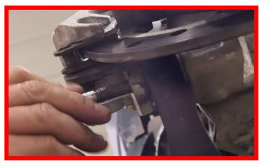
Next put the radius rod into the gusset plate side and hand tighten the bolts.
