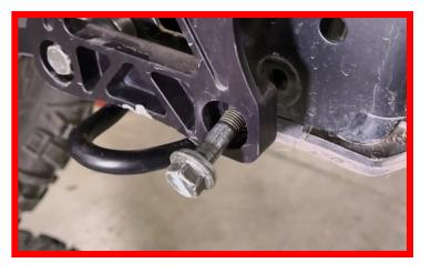
Using an 18mm Impact Wrench or Socket with Ratchet and End Wrench, remove the stock Radius Rod bolt from the Trailing Arm side. Next, remove the OEM Radius Rod. You will reuse the OEM bolts, nuts and washers so set those aside for use when reinstalling new ZBROZ Rods. NOTE: you do not need to remove the Gusset Plate.
