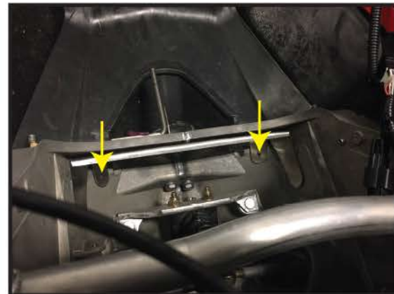
3. INSERT INTERNAL FRONT BRACE PLATE. CLAMP AGAINST FRONT STOCK CROSS MEMBER, DRILL (2) HOLES AND RIVET IN PLACE WITH .25" LONG STEEL RIVETS.
