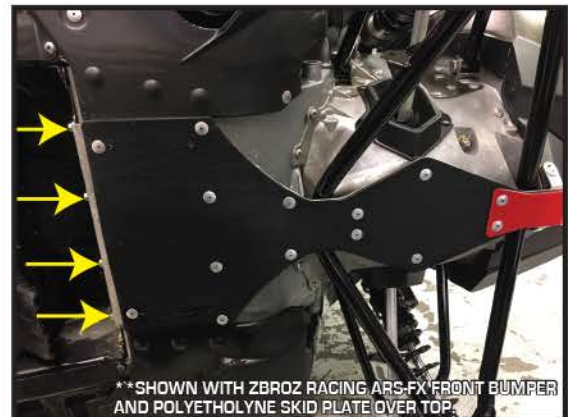
6. TURN SLED ONTO SIDE AND INSTALL SKID PLATE. UNBOLT AND REUSE (4) FACTORY BOLTS (SEE ARROWS). DRILL AND RIVET FRONT SIDE MOUNT USING (2) .75" LONG RIVETS TO POSITION SKID PLATE. THEN DRILL AND RIVET REMAINING (14) LOCATIONS USING .75" LONG RIVETS. **SHOWN WITH ZBROZ RACING ABS-FX FRONT BUMPER AND POLYETHOLYNE SKID PLATE OVER TOP.
