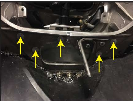
4. DRILL (5) HOLES INTO FRONT FACTORY MODULE AND THROUGH BRACE PLATE, THEN RIVET IN PLACE WITH .25" STEEL RIVETS..
