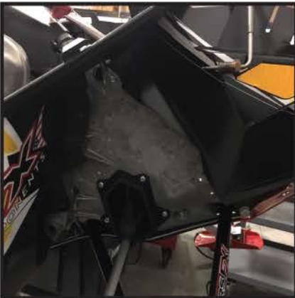
1. REMOVE HOOD, PIPE, SKI SHOCKS AND UPPER A-ARM FROM EACH SIDE OF BULK HEAD.
