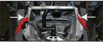
ATTACH BUMPER USING FACTORY BOLTS AND SUPPLIED (2) WASHERS AND (2) LOCK NUTS.
