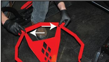
REMOVE STOCK BUMPER, REMOVE PIPE AND DISCONNECT PIPE SENSOR. ASSEMBLE ARSFX FRONT BUMPER TO SKID PLATE USING (2) SHORT RIVETS.
