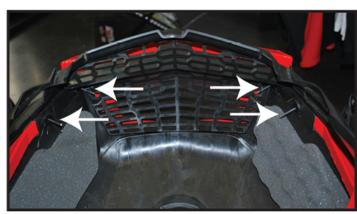
SLIDE BUMPER INTO POSITION AND ATTACH TO BULK HEAD USING (4) SHORT RIVETS THROUGH EXISTING HOLES FROM FACTORY BUMPER.
