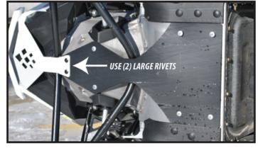
FLIP SLED ON SIDE, POSITION POLYETHYLENE SKID PLATE TO LOCATE AND DRILL OUT STOCK RIVETS. OVERLAP BUMPER SKID PLATE ON POLYETHYLENE SKID PLATE AND RIVET TO BULK HEAD USING (2) LARGE RIVETS. RIVET POLYETHYLENE SKID PLATE TO REST OF BULK HEAD USING (6) SMALL RIVETS.
