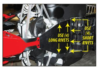
8. FINISH FASTENING POLYETHYLENE SKID PLATE USING (4) LONG RIVETS AND (4) SHORT RIVETS ALONG HEAT EXCHANGER.
