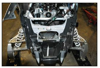
REMOVE HOOD AND SIDE PANELS. UNPLUG WIRE HARNESS. REMOVE PIPE SENSOR AND PIPE. USE 10MM END WRENCH, 10MM SOCKET AND T40 TORX TO REMOVE OEM BUMPER.
