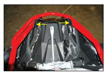
ATTACH TOP FRONT OF BUMPER USING THE (2) OEM T40 TORX SCREWS.
