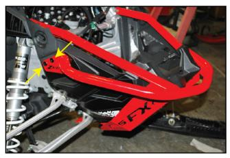
5. POSITION SIDE UPPER TABS OF ZBROZ RACING BUMPER ALONG SIDES OF BELLY PAN. DRILL HOLES THROUGH BULK HEAD AND FASTEN WITH (2) SHORT RIVETS ON EACH SIDE. USE THE (4) RIVET BACKWASHERS ON THE INSIDE.
