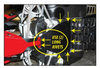
POSITION POLYETHYLENE SKID PLATE, ALIGN WITH THE (8)
