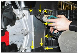
FLIP SLED ON SIDE, POSITION AND LINE UP POLYETHYLENE SKID PLATE TO THESE (8) OEM RIVET LOCATIONS. REMOVE POLYETHYLENE SKID PLATE AND DRILL THROUGH TO REMOVE THESE (8) OEM RIVETS.
