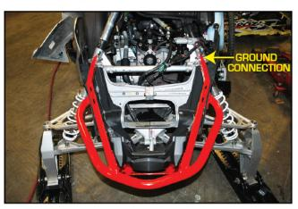
3. SLIDE ZBROZ RACING BUMPER INTO PLACE AND FASTEN WITH OEM HARDWARE.
