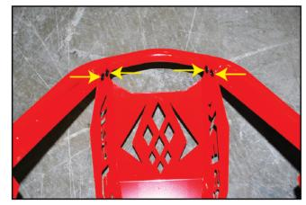
2. ASSEMBLE ZBROZ RACING FRONT BUMPER TO SKID PLATE USING (2) SHORT RIVETS ON EACH SIDE.
