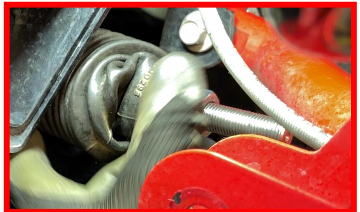
Locate and insert the reducers. The shorter "hat shaped" reducer goes into the top and the longer reducer goes into the bottom side. NOTE: the tapered end of the longer reducer inserts into the wheel hub mount side.
