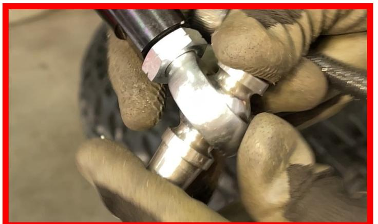
Insert the supplied 12mm bolt and Nut down through with the nut on bottom. Torque supplied bolt to factory specs.
