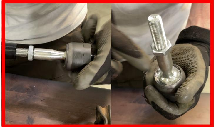
Slide the factory boot over the new ZBROZ Axle Rod exposing the Jam Nut.
