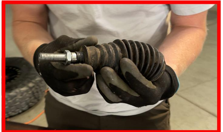
Reconnect the Axle Rod with boot to Billet Tie Rod Assembly.
