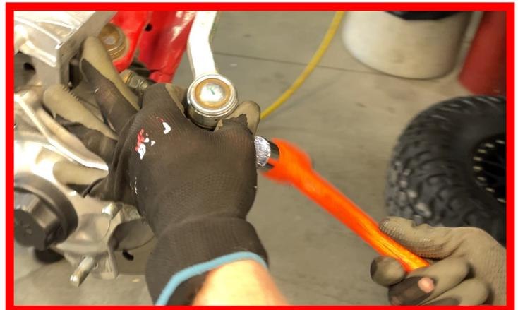
Remove the Axle Joint from the frame side connection using a large Crescent Wrench.
