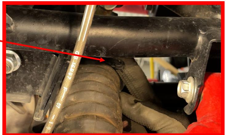
Remove the Tie Rod Bolt from the Spindle. NOTE: you may need to use a Hammer or Mallet to tap up on the bolt to dislodge it free.
