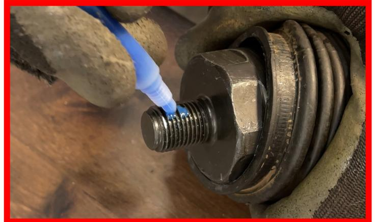
Thread the Axle Rod side into the PRO XP Frame. A trick to get it started is leaving the rod disconnected from the Axle Rod side. This will help make sure it is not cross threaded. Finish tightening with a large Crescent Wrench to factory torque specs.
