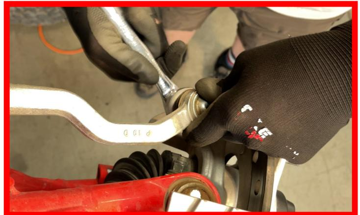
Remove the Zip-Tie holding the Tie Rod Boot in place located on the frame side. Slide the boot down exposing the Axle Joint.
