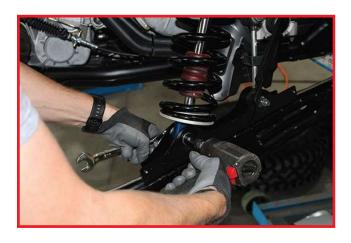
Set "zero Preload" by pressing down on trailing arm and holding the shock to full internal bump stop spring. Rotate preload ring clockwise until spring stack contacts preload ring. (That is zero pre-load)
