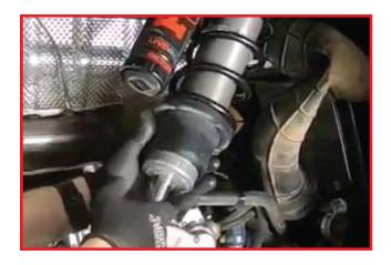
Install new main spring and OEM lower spring retainer in reverse order of how it was removed.
