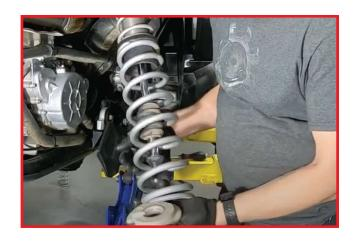
Install new large rear billet cross over ring. Loosen the allen screws with a 3/32" allen wrench. Do not loosen allen screws all the way out.
