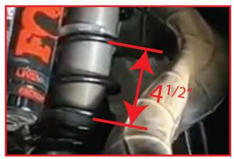
Align or clock lower coil end of new tender spring to upper coil end of new main spring.
