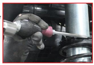
Rotate OEM preload rings counter clockwise all the way to top of threaded shock body. OEM spring stack should now be loose.
