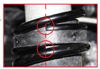
After preload is set and while shock is full extended positon cross over ring so that there to 1" gap between bottom edge of cross over ring and top edge of spring divider. Tighten allen screws.
