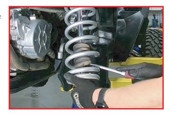
Rotate OEM spring stack and preload ring counter clockwise to the top of the threaded shock body. Loosen the ACC pre-load off of the spring stack
