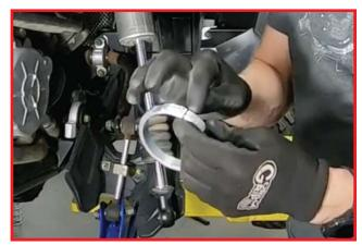
Starting at the bottom of the threaded shock body, rotate the cross over ring counter clockwise up the threaded shock body. Be careful not to cross thread and damage cross over ring or shock body. Set cross over ring 6" from shock body cap. Do not tighten cross over ring, it will need to be moved once preload is set.
