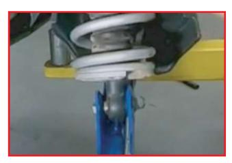
Push up on spring stack to remove OEM lower spring retainer. As shown ---->
