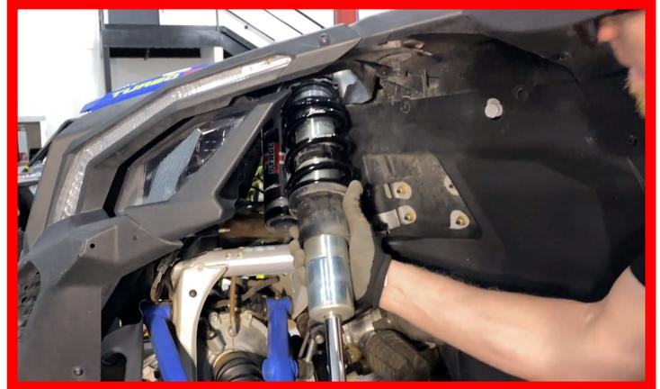
Now slide the NEW ZBROZ Main Spring onto the shock body all the way up to the Spring Divider.
