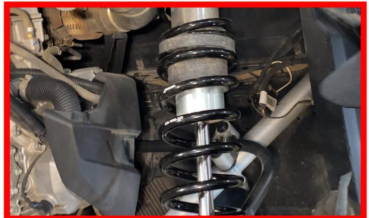
Next Place the lower Spring Retainer back on the same way it came off and then mount your shock back to the Trailing Arm with the lower shock bolt. Tightening the nut and bolt to factory torque specs.
