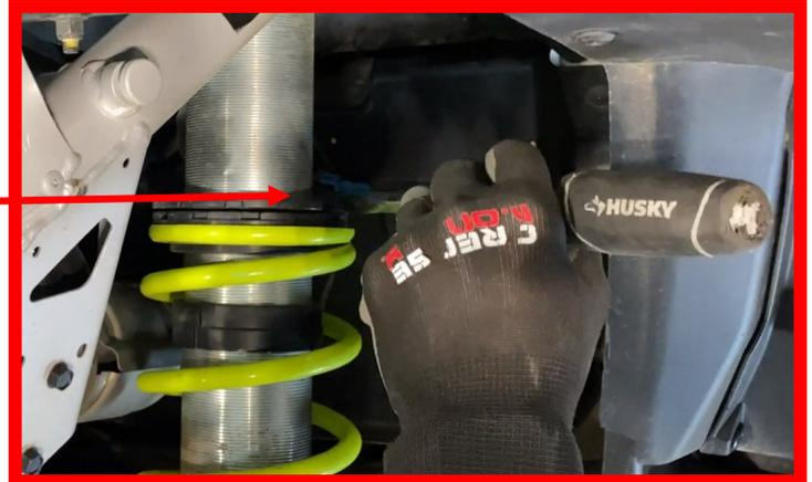
Loosen lower shock bolt on the A-arm. Do not disconnect it from the Trailing Arm at this time.
