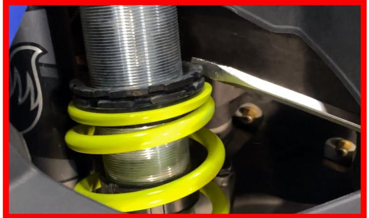
Now back the preload off by grabbing the Spring Stack and rotating it counter clockwise to fully loose.
