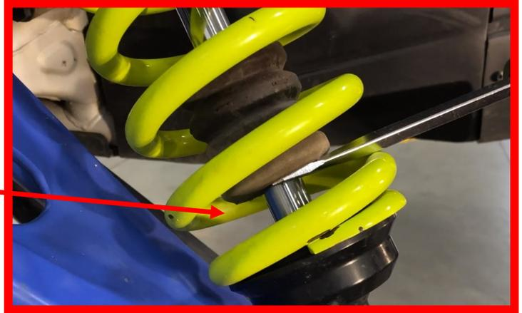
Loosen lower shock bolt on the A-arm. Do not disconnect it from the A-arm at this time.
