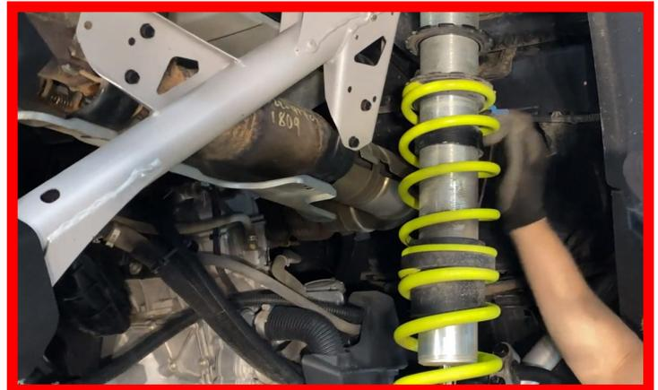
Remove the bottom retainer with guard by lifting up on the Spring Stack providing enough clearance to remove the retainer.
