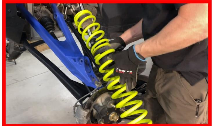
Take the new ZBROZ Tender Spring and place it back on top of the Spring Divider the same direction it came off and slide them back up to the top of the shock body.
