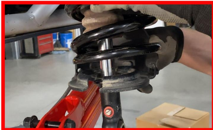
Turn your Cross-over nut down until it is half-way down the inside of your Tender Spring. In order to set a true zero preload point make sure the shock is fully extended. You will have to push down on the wheel hub to extend the shock.
