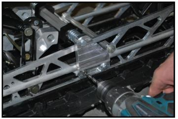
4. USE 5/8" DRILL BIT TO MAKE SPACE FOR BOLT TO CLEAR ON SKID RAIL.
