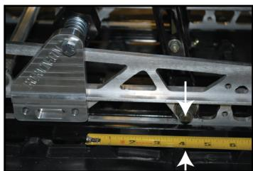
2. POSITION K.I.S.S. COUPLER ASSEMBLY 4" BACK FROM BOTTOM SCISSOR ARM BOLT MOUNT LOCATION.
