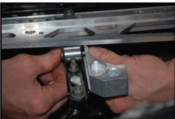
1. INSTALL IMPACT BLOCKS TO EACH SIDE OF THE SCISSOR ARM USING THE SUPPLIED SPACERS AND PAN HEAD BOLTS.
