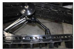
LAY SLED ON SIDE. REMOVE CROSS SHAFT BOLTS USING 8MM ALLEN WRENCH.
