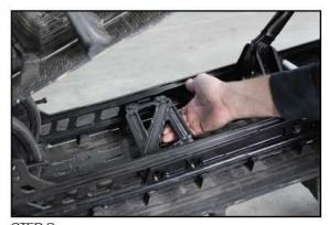
STEP 3 INSTALL BILLET Z-BRACE. LOOSEN REAR AXLE BOLT, AND LOWER SCISSOR PIVOT BOLT. INSERT Z-BRACE, ALIGN HOLES AND TIGHTEN WITH (2) Z-BRACE BOLTS.
