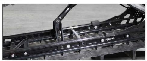
STEP 4 INSERT CROSS SHAFT USING OEM BOLTS (DO NOT USE OEM CROSS SHAFT WASHERS) AND TIGHTEN. TIGHTEN REAR AXLE BOLT AND LOWER SCISSOR PIVOT BOLT.
