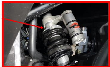
Take a measurement from the top of the Tender Spring down to the bottom of the lower Main Spring. This should be about 15 1/2".
