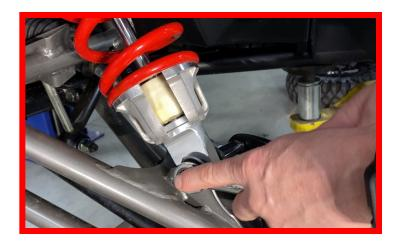
Using a flathead screwdriver raise the Bump Stop up above the retainer.
