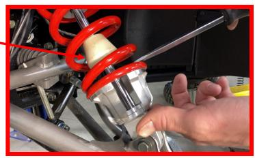
Next, loosen your pre-load all the way down until the collar is all the way to the top.
