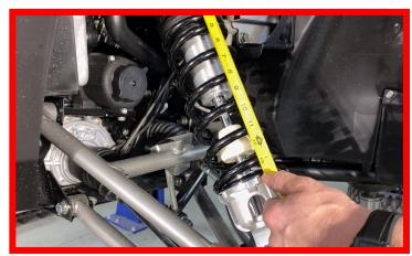
\*Additional Preload may be needed depending on after-market accessories (bumper, cage, tire carrier, stereo system). You can put more pre-load on by repeating turning the pre-load nut more.
