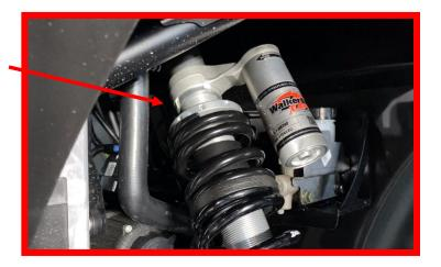
Take a measurement from the top of the Tender Spring down to the bottom of the lower Main Spring. This should be about 13 3/4".
