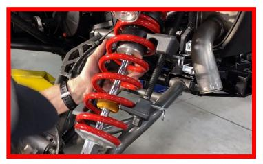
Now remove the lower shock bolt and swing it away from the Trailing Arm. Slide the spring stack down to completely remove it from the shock body.
