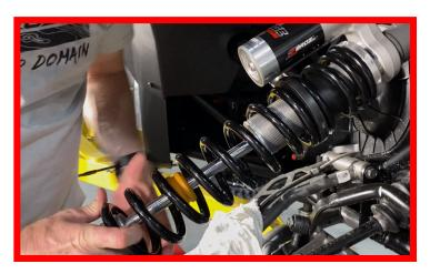
Using the Strut Compressors again, clamp and compress your ZBROZ Main Spring enough to slide the OEM Spring Retainer back on. After the Spring Retainer is secure, remove the Strut Compressors.
