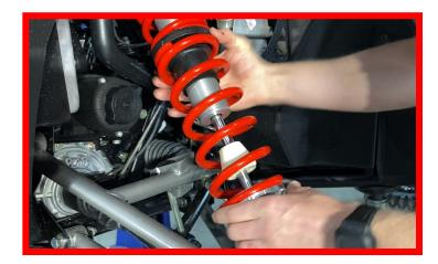
Remove the bottom retainer by lifting up on the spring stack with the help of another person or by using a Strut Compressor tool.
