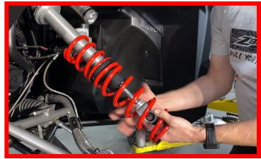
You will now need to cut the OEM Spring Divider 1/4" down from the long end. Using a measuring device mark 1/4".
