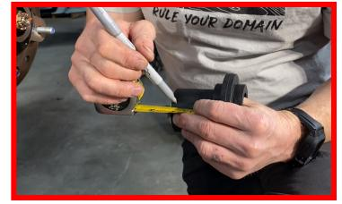
Install OEM Spring Divider with long end pointing up into the new ZBROZ Tender Spring.
