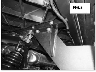
• Attach the Mounting Bracket to the previously installed threaded inserts (see Step 2) in the bottom of the square tube frame with the included (2) 8mm x 30mm Hex Bolts, (1) 8mm Lock Washers and (2) 8mm Flat Washers, (Figures 5 & 6). Do not fully tighten hardware at this time. Repeat Steps 1—5 to install the passenger/right Mounting Bracket. NOTE: Pull clips from side of frame attaching wiring harness, (Figure 7). Once Bracket is installed, snap clips into top plate on Bracket, (Figure 8).
