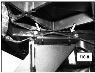
With assistance, hold the Rear Bumper assembly up to the inside of the Mounting Brackets. Temporarily support the weight of the Bumper. WARNING: To avoid possible injury or damage to the vehicle, do not proceed until the Bumper is fully and safely supported. Attach the Bumper to the inside of the Mounting Brackets with the included (4) 10mm x 30mm Hex Bolts, (8) 10mm Flat Washers, (4) 10mm Lock Washers and (4) 10mm Hex Nuts, (Figures 9 & 10). Snug but do not fully tighten hardware at this time.
