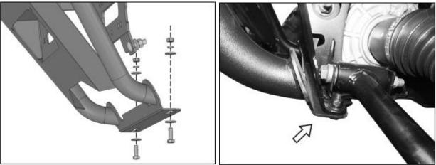
• Level and adjust the Front Bumper and fully tighten all hardware.
