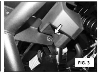
• Attach the bottom mount on the Bumper to the bottom of the frame with the included (2) 8mm x 25mm Hex Bolts, (4) 8mm Flat Washers, (2) 8mm Lock Washers and (2) 8mm Hex Nuts.
