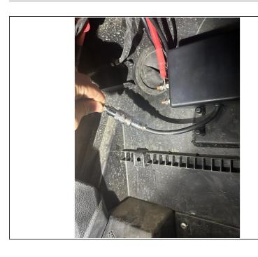
Determine where you would like to operate the remote in vehicle and route provided USB cable to the solenoid. (Image 1)Connect cable to pigtail on solenoid.
